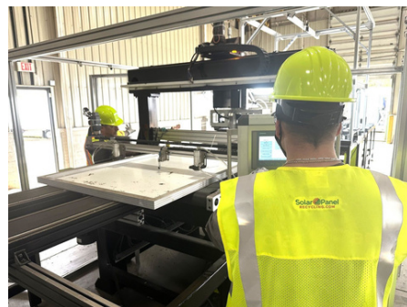
Figure 2 (left): Removal of Aluminum Frame and Electronics from a Solar Panel
