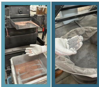
Figure 4: Copper powder (left) and Silver-Silicon mixture powder (right) after Step 4
